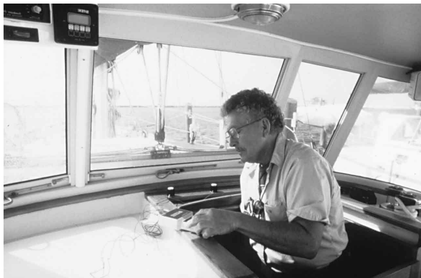
Fig. 1. Pest control operator using the acoustic emissions detector on wood trim in a boat to detect drywood termites.
